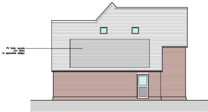
west elevation (side)
